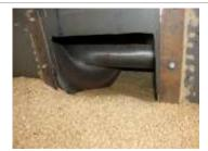
2. Bad idea. You can slip and slide right into the exposed shear points on this floor auger.
