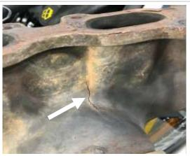
Warning! Cracks in vehicle exhaust manifolds (see arrow) can allow harmful carbon monoxide (CO) gas to enter the engine compartment and flow into the cab through the ventilation system. Photo: L&I
