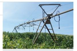
Field irrigation systems, as shown in this photo, are large metal structures that can span 1,200 ft and are often powered with 480 volts.
