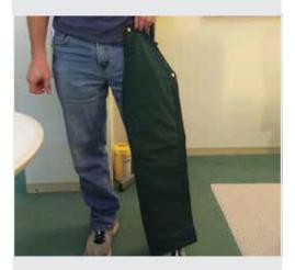
Contact with moving chain saw teeth can cause poorly secured Kevlar safety inserts like these to roll sideways or up inside of jeans, leaving legs vulnerable to deep cuts.
