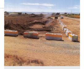
Driving farm equipment too close to manure storage areas can result in tip overs with fatal consequences. Concrete blocks and other types of barriers can prevent this.
