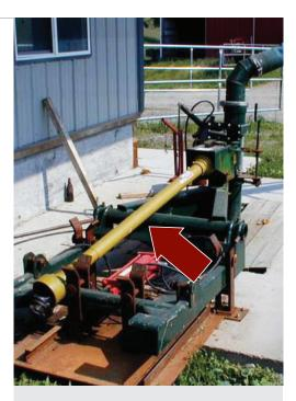
Exposed and spinning shafts used to operate manure pumps have the power to kill and maim. The shaft shown is covered by a safety shield (see arrow).
