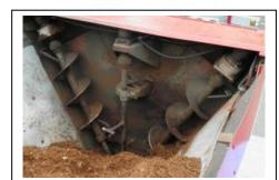
Danger zone! Do not enter the hopper or use hands or any part of your body to clear jams or move materials. Even slow-moving mechanical parts like the rotating shaft and augers shown here, have killed or maimed workers that entered hoppers.
