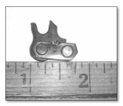
A small size but a deadly threat: chain shot from harvester or processor heads and stroker-log merchandisers or delimbers can maintain lethal velocity after penetrating 1/2-inch thick polycarbonate windshields.
