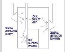
For better ventilation: the direction of air flow should move from a clean area (customer counter) to one that's less clean (machine area) where vapor is captured and vented outdoors by local exhaust and a wall-mounted exhaust fan.
