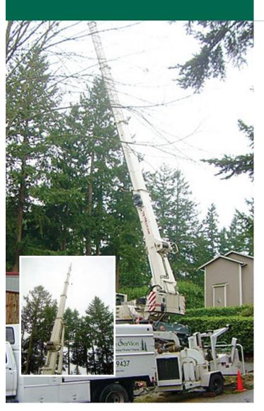
A tree trimmer suspended from the hook of a crane was killed when his line detached, dropping him more than 70 ft to the ground below.
