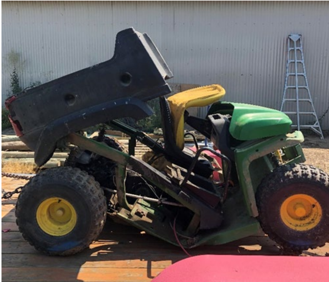
Photo 1. Utility Task Vehicle (UTV) with collision damage caused by passenger car.
