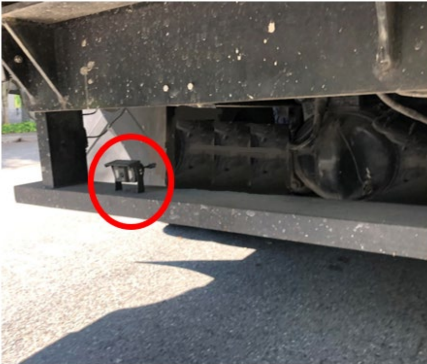
Photo 4. Backup camera mounted on dump truck after the incident.
