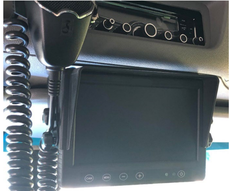
Photo 5. Backup camera monitor in truck cab installed after the incident.
