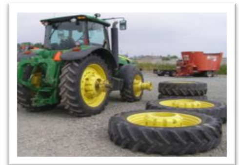
A mechanic was removing unsupported tires when one fell on him.
