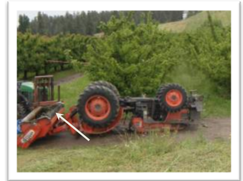
Some attachments can change the center of gravity making the tractor easier to tip and roll over.
