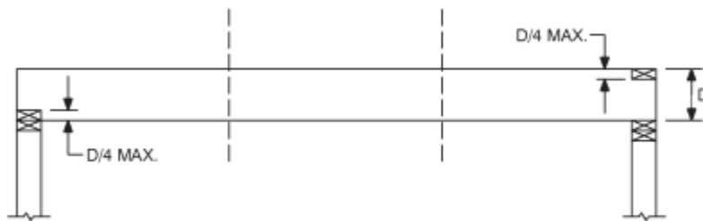
FLOOR JOIST—END CUTS
