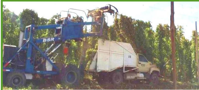
Top-cutter harvester machine cutting hop vines that then drop onto a truck. The photo was taken at the incident hop yard.
