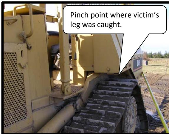
Pinch point between track and fender where the victim's left leg was caught and crushed.
