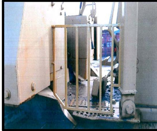
The employer added this barrier to restrict the operator from exiting on the right side. The parking brake is in the “down” position preventing the machine from moving. The operator can now safely exit by the left side of the cab. If the parking brake is not set the lever is in the “up” or horizontal position which restricts the operator’s path of exit from the left side of the cab, thereby serving as a reminder to set the parking brake.
