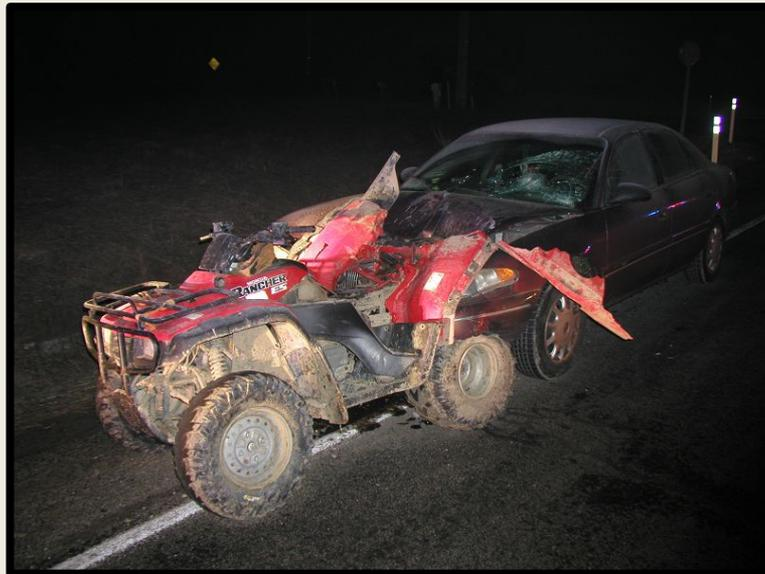
Photo of incident scene where a shepherd died when he was operating an ATV on a highway at night and was struck from behind by a passenger vehicle. It was reported that the ATV's tail and brake lights were not working.
