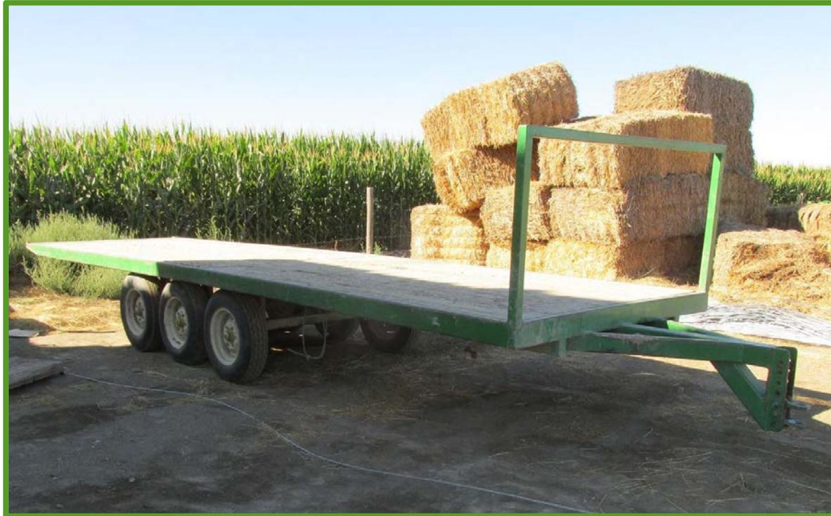
Twenty-five foot flatbed trailer that detached from the tractor and landed on top of the tractor, crushing the operator.
