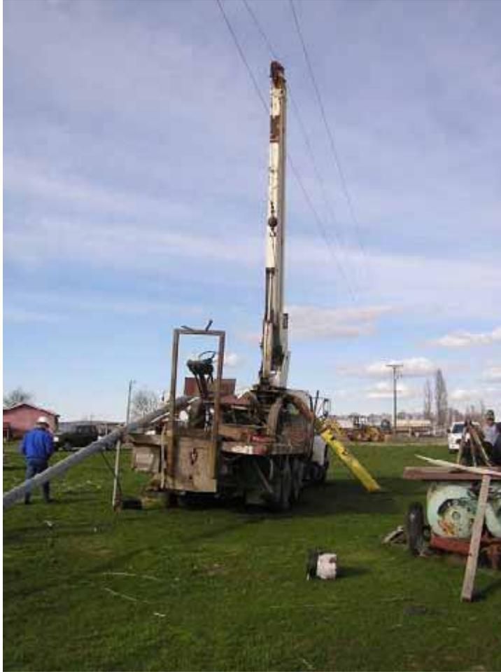
**Photo:** The crane and site after the incident, showing the boom arm in contact with the high-voltage line.
