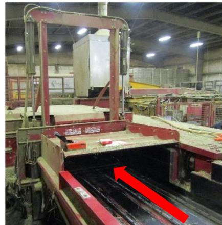
Incident hay press showing the area where the victim was working when he was struck by the guillotine blade.
