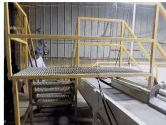
Staircase platform that was being moved by a forklift shown after the incident placed over a potato conveyor.
