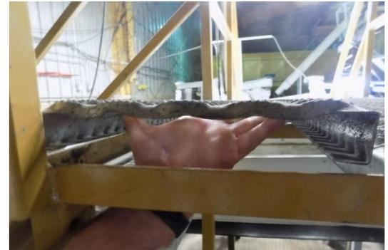
When the staircase platform fell off the forklift forks, a metal decking panel, like this one, came off the platform and struck the victim's head.
