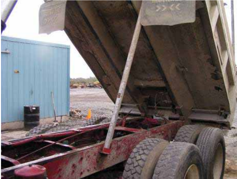
Figure 1. The truck after the incident with the bed raised and safety pole in place.
