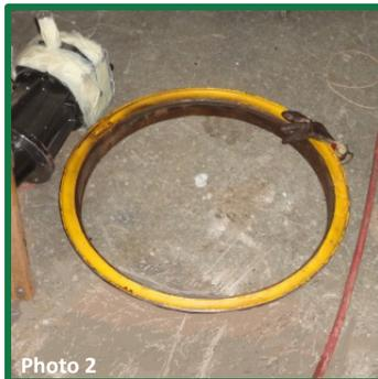
**Photo 2:** Larger of two rings that separated from rim assembly and struck worker.
