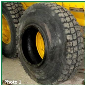
**Photo 1:** Blown-out road grader tire that injured worker was attempting to inflate when explosive separation occurred.
