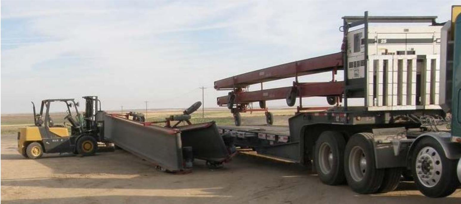
Stacked conveyor belt tables that fell from the trailer and struck the victim as he was laying out tie-down equipment. A witness used the forklift to raise the tables off the victim.
