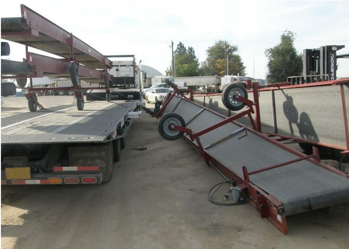
Rear view of stacked conveyor belt tables that fell from the trailer and struck the victim. (The tables remaining on the trailer were tied down post-incident for safety.)
