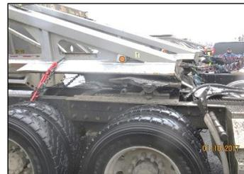
Belly dump trailer's king pin and the truck's 5<sup>th</sup> wheel plate after the incident.
