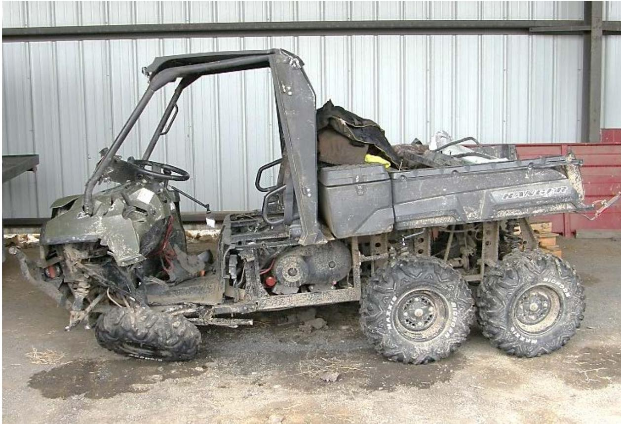
UTV after the incident showing the damaged left front that was struck by the pickup truck.
