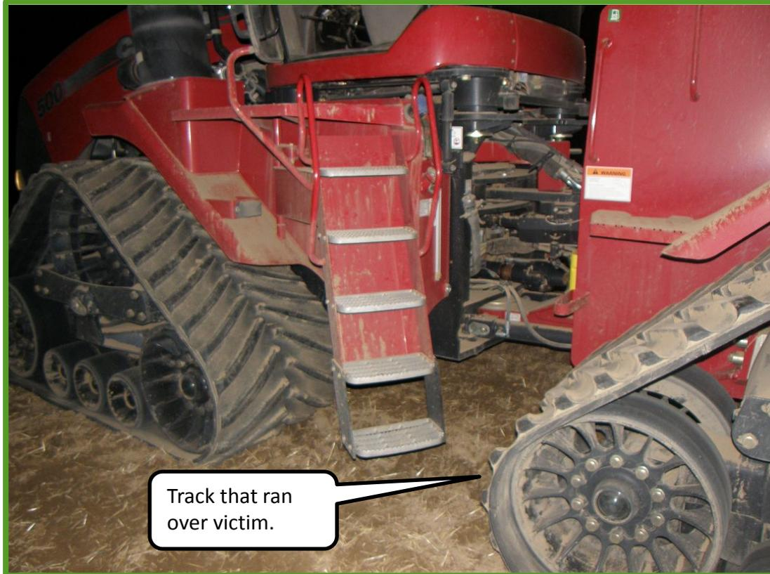
Incident scene where the victim attempted to climb the tractor's cab access ladder and was run over by the moving left rear track.
