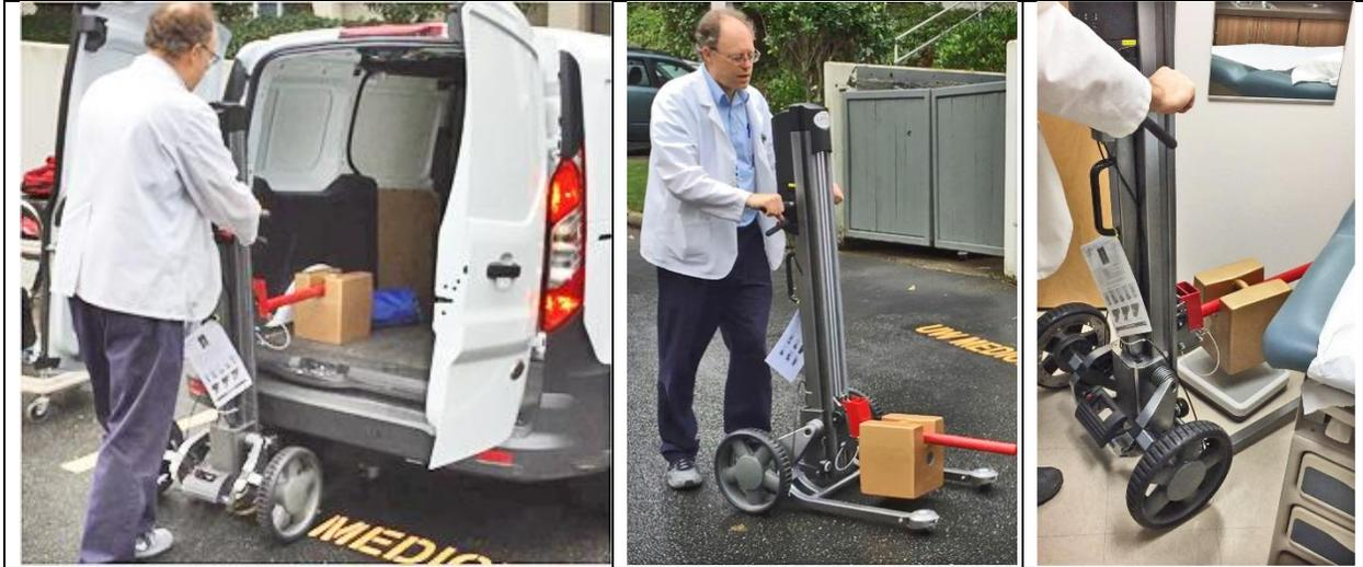
Department employees came up with the idea to get a single unit 100 kg calibration weight. It is safer and less precarious to roll one large, heavy weight from place to place with the lifting device instead of 10 smaller weights.
