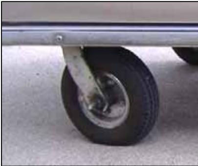
This was the second caster tried. The tires would sink and grab at the ground or floor covering. This resulted in push and pull forces that exceeded recommended limits.
