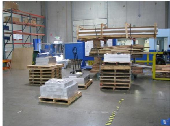
The in-house maintenance department fabricated three pairs of various sized sawhorses. The sawhorses created standing workstations that significantly reduced awkward postures and contact stress.
