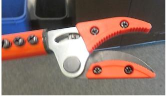
After the incident, the company trained employees to initiate an emergency stop before clearing an obstacle from an LGV's path, and to use a long-handled snipping tool to remove plastic stringers instead of reaching or bending under the forks of the LGV.
