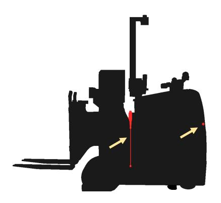
Diagram indicating the location of the emergency stop button and rope pull. An identical set was present on the other side of the LGV.
