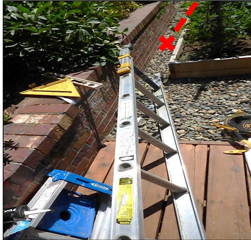
**Photo 1.** Base section of the ladder showing where it was set up behind a wood-framed garden bed (shown by “X”) and leaned against a house chimney chase at a 65- degree angle.
