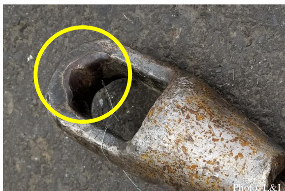
Photo 6. Socket was taken out of service due to greater than 10% wear.
