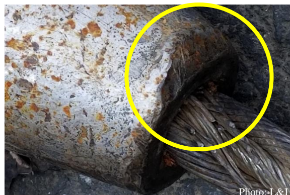
Photo 7. Pitting on socket is an indicator or broken wires
