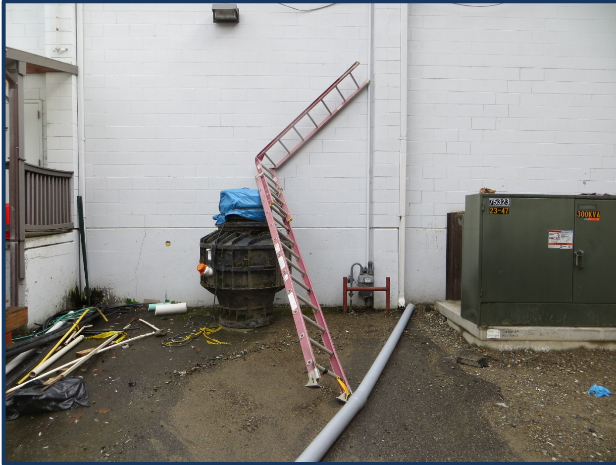
Incident scene showing the broken 24-foot, fiberglass extension ladder from which the laborer fell 12 feet.
