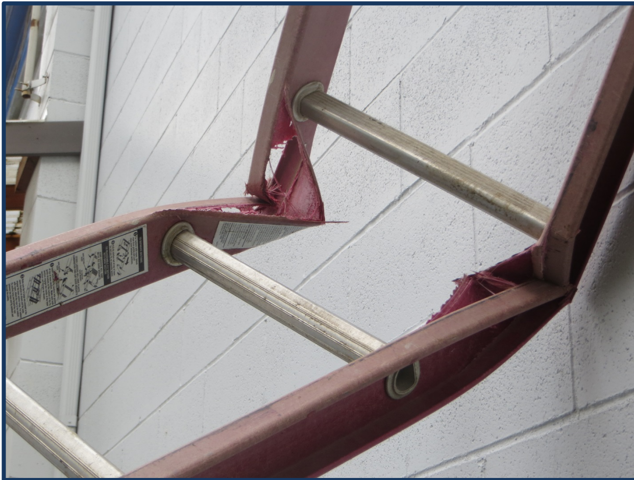
Ladder at incident scene showing the broken, bent rails.
