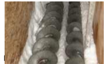
spaces with exposed double-screw conveyers until you verify the equipment has been properly locked and tagged out.
