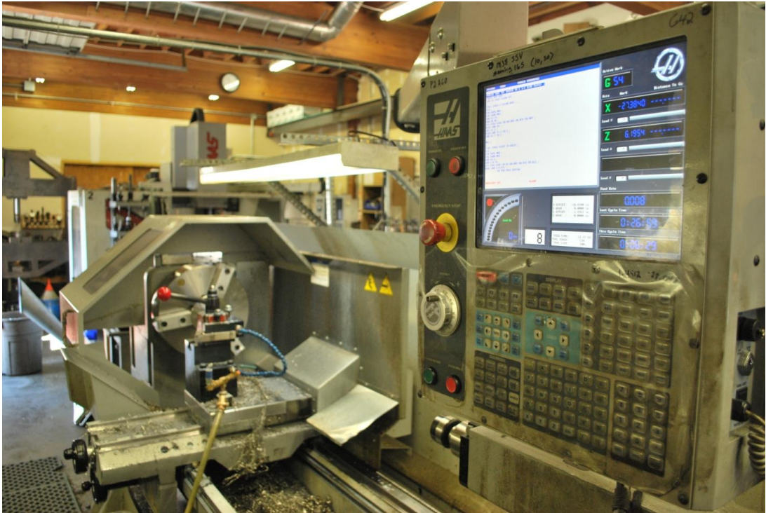
Photo 2. HAAS TL-3W lathe bed, control panel, cutting head, and chuck
