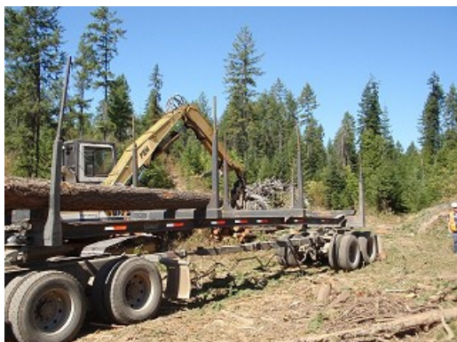
Photo 1: “Turkey rack” trailer intended for hauling loads of short logs
