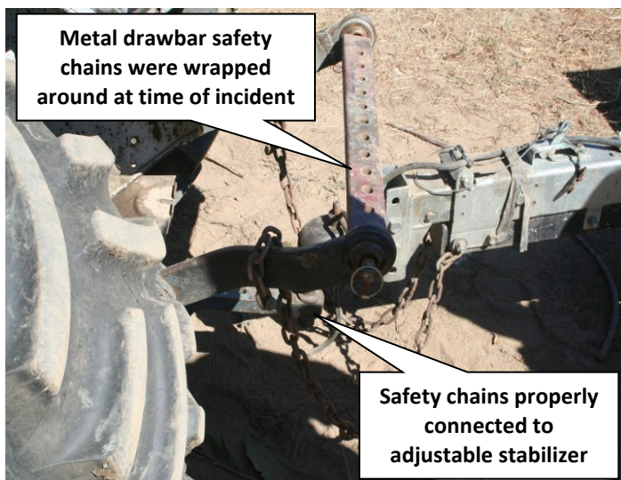
Photo 7. Example of employer's procedure for properly connecting safety chains to stabilizer arms, not the metal drawbar.
