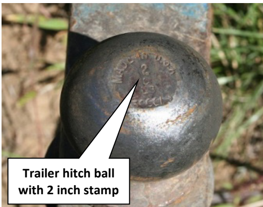
Photo 3. The 2 inch trailer hitch ball that was mounted on the bumper pull hitch and connected to the trailer coupler
