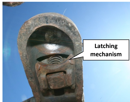
Photo 6. Inside of 2 5/16 inch trailer coupler showing latching mechanism and screw used to secure coupler to trailer hitch ball
