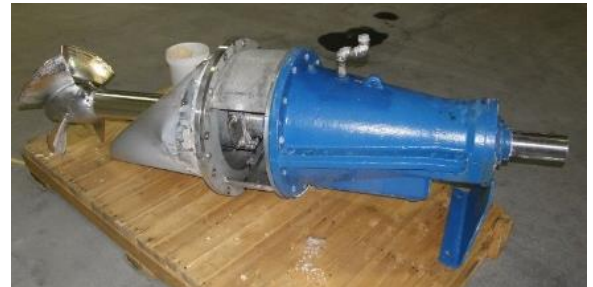
Photo 1 Recirculation pump, removed from housing.
