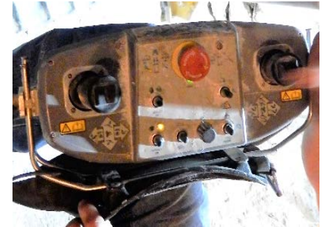
Photo 1: Remote control box with red emergency stop button.
