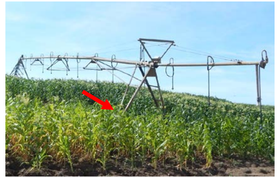
A wheel at the base of the irrigation system's tower ran over and crushed the operator.
