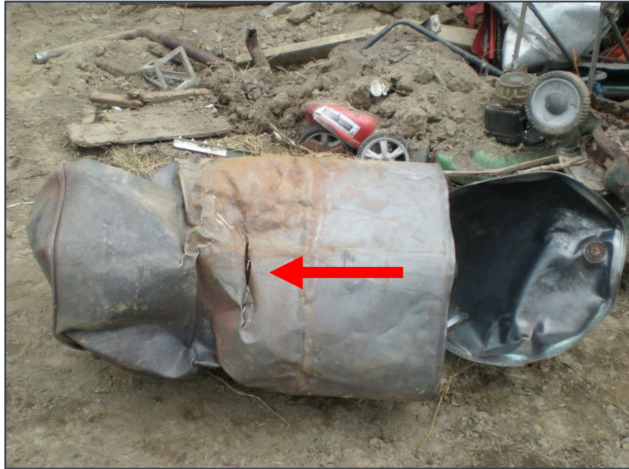
Photo 1. Cut made by victim on 55-gallon drum before it exploded.
