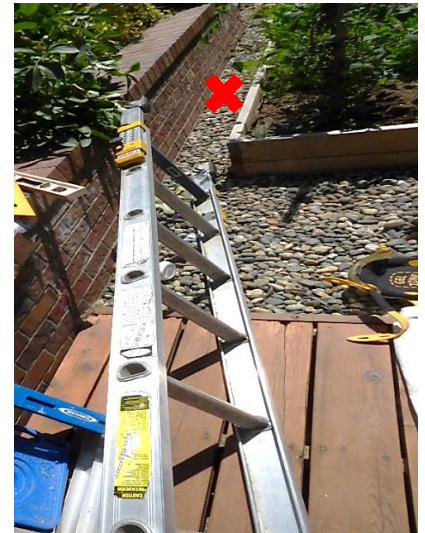
Base section of ladder and location it was set up (X) and leaned against the chimney chase at a 65-degree angle.
