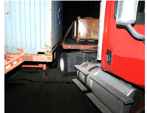
Pinch point between the two trailers where the truck driver was crushed when his semi-truck and trailer rolled backward.
