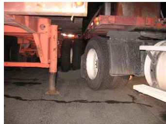
Close up of pinch point between the two trailers where the driver was crushed.
