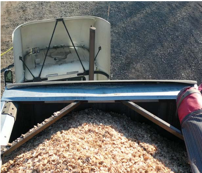
Photo 5: Driver’s trailer with manual tarping system missing the elastic stretch cord across the top end cap at front of trailer.
