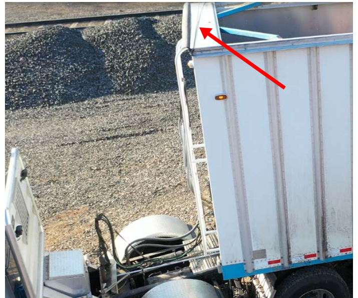
Photo 6: Tractor-trailer that stopped near the incident scene. Arrow points to intact elastic stretch cord across the top end cap at front of trailer.
