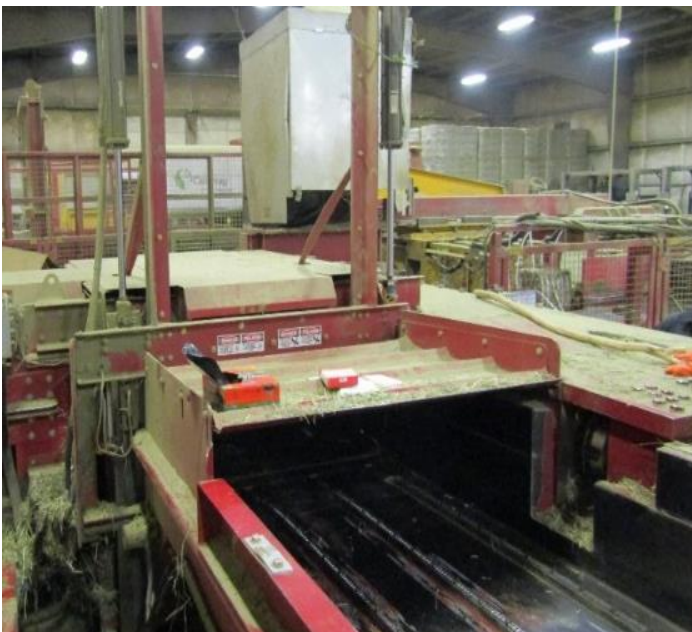
Photos 4 and 5: The left photo shows the hooded intake opening of the main press where the machine's scale pan, steel guillotine, compress chamber, and ejection device are located. The right photo shows a steel guillotine blade of the same type that struck the operator inside the main press.
