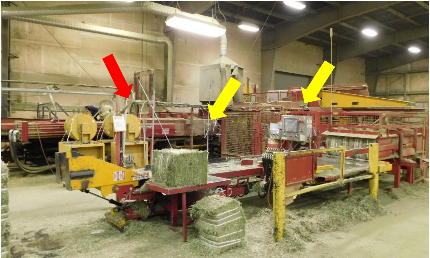
Photo 10: Red arrow shows the location of the guillotine where the operator was found. The yellow arrows show the locations of red emergency stop (E-Stop) buttons at the main press and operator's station.
