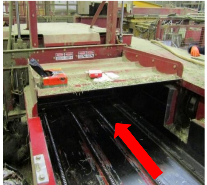
Photos 7 and 8: The left photo shows hay press after the incident showing hay bales on the machine's conveyor. The left photo shows where the operator crawled into the hooded intake opening of the main press to push hay bales through in order to prepare the machine for scheduled maintenance.
