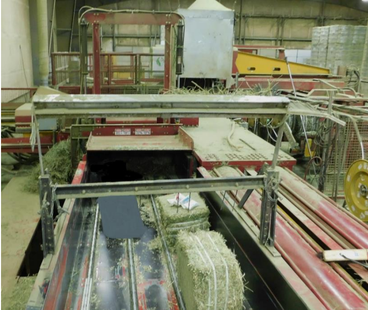
Photos 7 and 8: The left photo shows hay press after the incident showing hay bales on the machine's conveyor. The left photo shows where the operator crawled into the hooded intake opening of the main press to push hay bales through in order to prepare the machine for scheduled maintenance.
