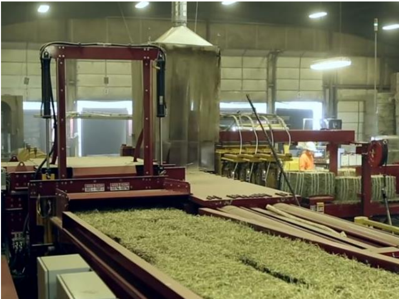
Photo 2: Chain-driven conveyor moving field baled hay into the machine's main press that processed them into smaller compressed cubes for shipping to customers.
