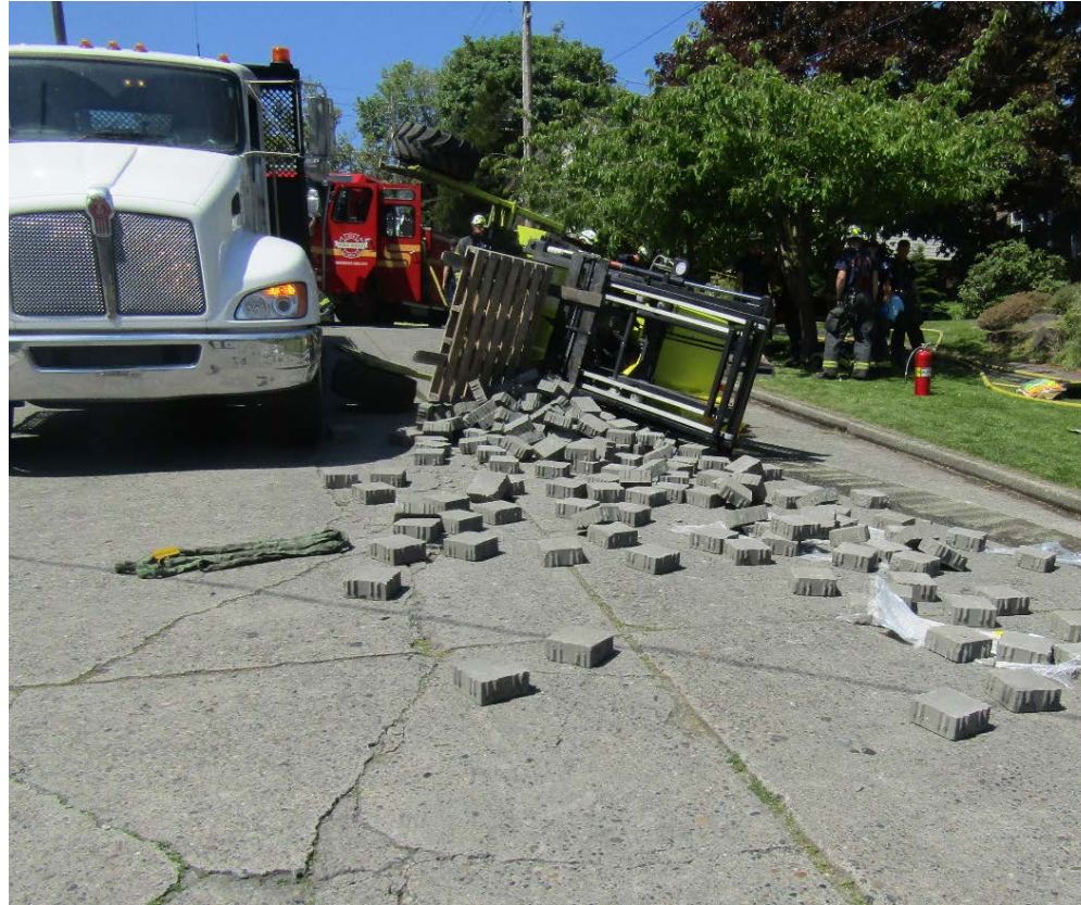
Photo 2. Overturned forklift showing city street slope and surface.
