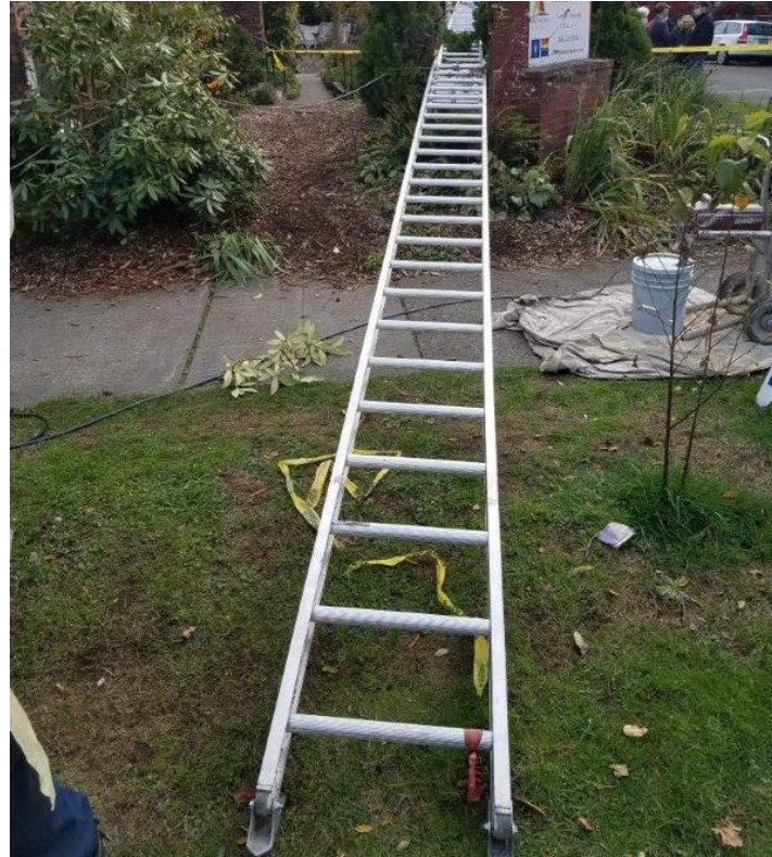
Photo 4. The 48-foot aluminum extension ladder that contacted the overhead power line.
