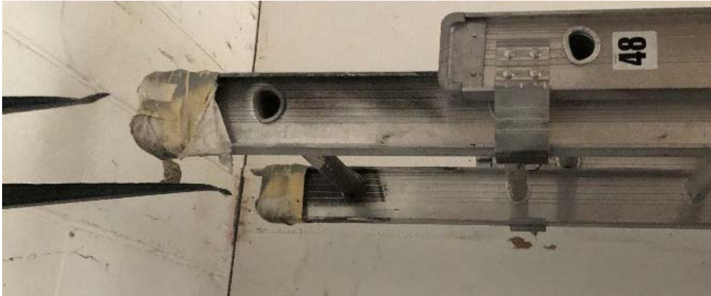
Photo 5. Top of the extension ladder showing burn marks where the ladder contacted the power line.
