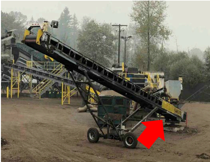
Photos 2 and 3: Left photo shows front side view of radial stacker conveyor involved in the incident. Right photo shows rear side view of stacker. Red arrows show the conveyor's tail end location where the lead screen plant operator was pulled in between the return idler roller and conveyor belt.
