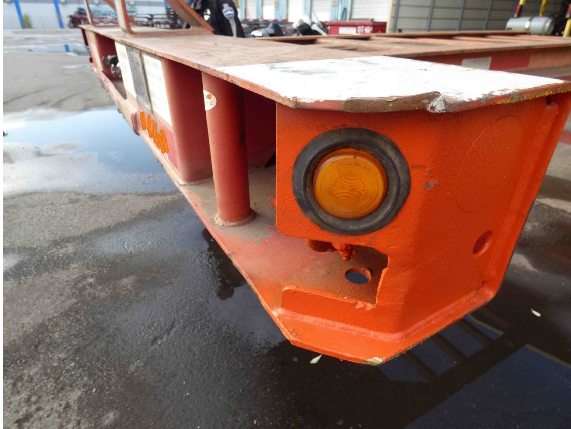
Photo 5. View of damage to the front of the trailer where it was hit by the rollaway semi-truck.
