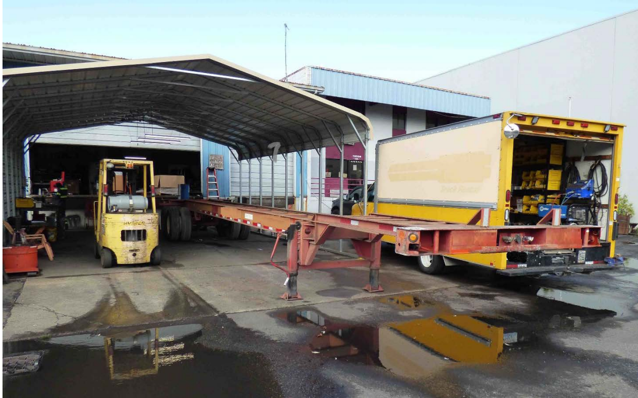
Photo 2. View showing outdoor repair area and front of the trailer that was hit by the rollaway semi-truck. The impact pushed the trailer off its jack stands toward the mechanic working behind it, crushing him against a large steel bumper jack.
