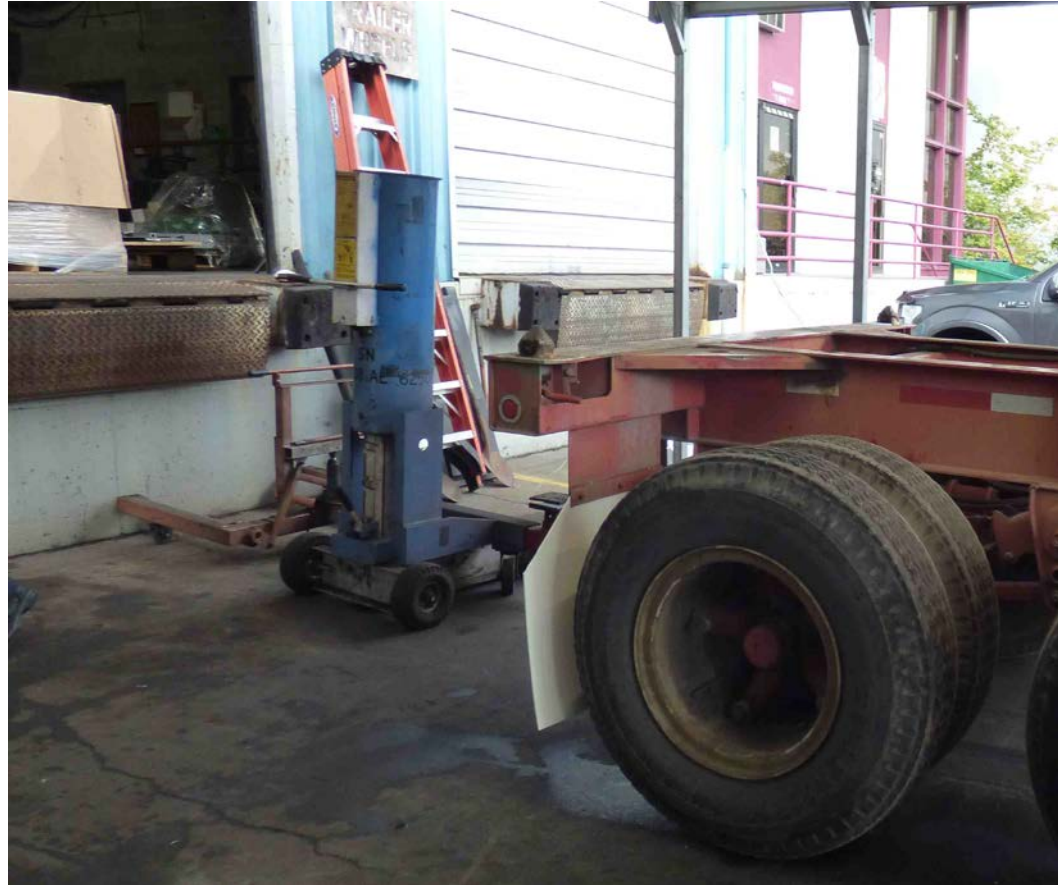
Photo 3. View of loading dock and blue steel bumper jack behind the trailer that crushed the mechanic.
