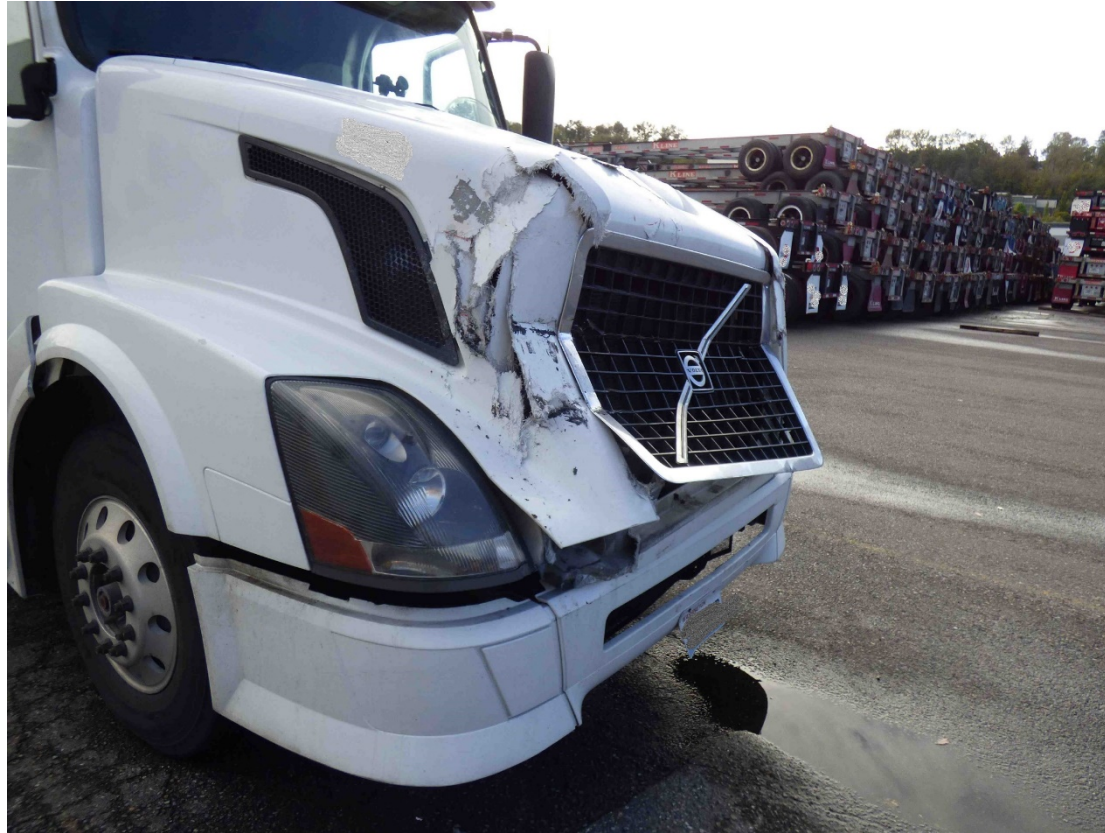
Photo 6. View of damage to rollaway semi-truck's fiberglass engine hood that resulted from hitting the trailer that crushed the mechanic.
