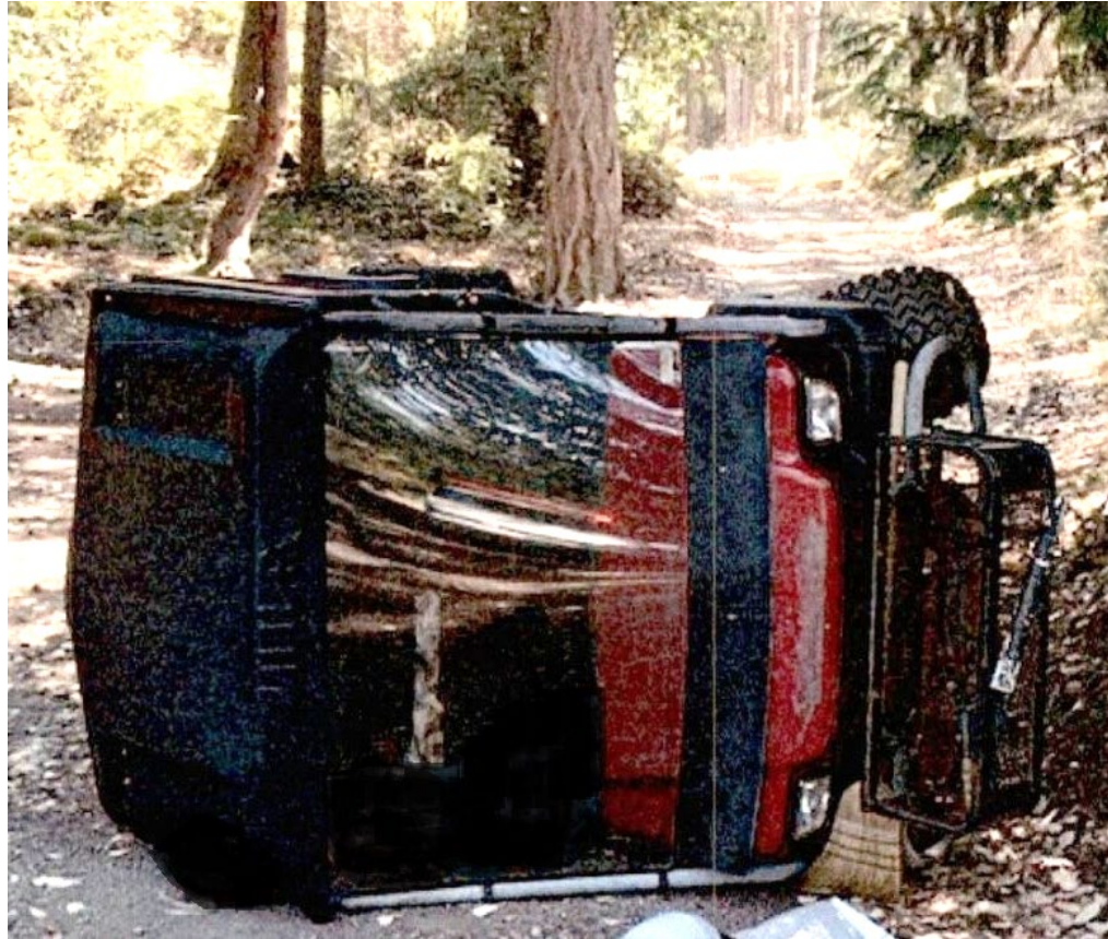
Photo 2. Incident scene showing UTV overturned on its passenger side. The unrestrained groundskeeper was ejected from her seat, pinned and crushed under the cab frame/rollover protective structure (ROPS).
